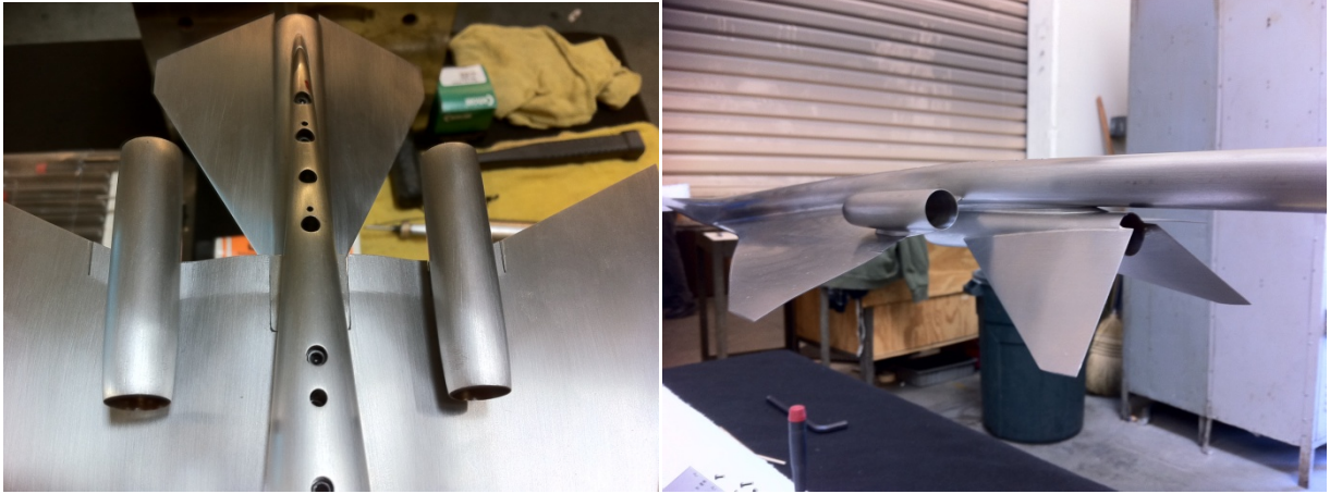
Figure 67. Difference between model aft fuselage design (blade support) and aft sting support
