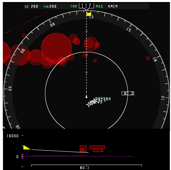
Figure 11: Prototype Navigation Display of Weather Hazard Cylinders
