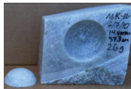
Figure 2. Photograph of Soapstone Sample (left) cut from parent rock (right) by the Rockballer prototype; the sample is 14.8 mm deep and has a mass of 26 grams.
