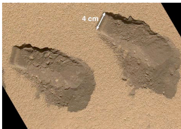
Figure 4. A view of the 3 rd (left) and 4 th (right) trenches made by the scoop at Rocknest in October 2012 acquired by MAHLI on Sol 84. The upper surface of the drift is covered by coarse sand grains approximately 0.5-1.5 mm in size. These coarse grains are mantled with fine dust. Beneath the surface is finer sand, which is darker brown. The left end of each trough wall shows alternating light and dark bands, indicating that the sand inside the drift is not completely uniform.
