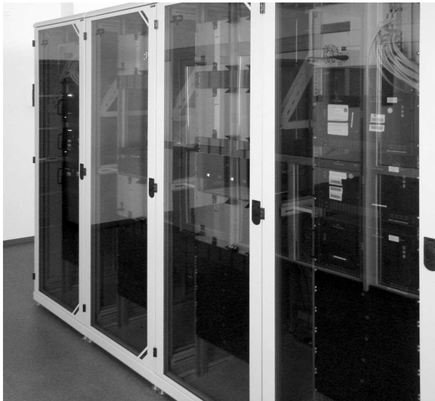
Figure 1. View of the six-station ARC correlator, showing four racks containing (left to right) signal distribution and synchronization system (SDSS) and three Mark 5B playback units, two correlator crates and KVM, three correlator crates, and one more cabinet with SDSS and three Mark 5B playback units.
