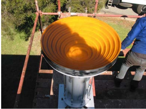
Figure 2. 15-m XDM's S/X receiver package looking at sky during noise temperature tests. (Credit K. Jones)
