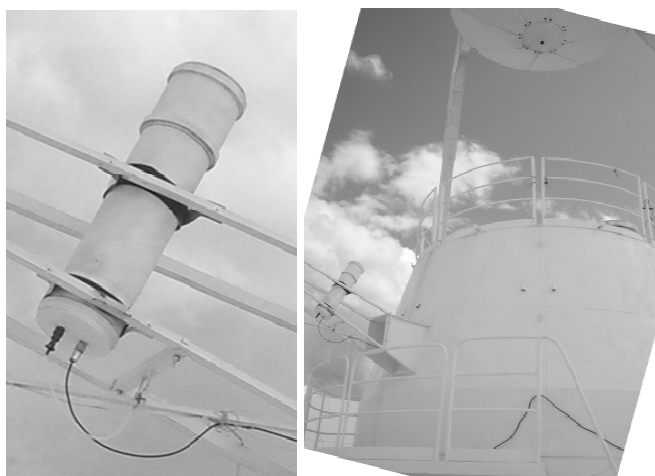
Figure 5. The breadboard model of the broadband phase calibration system mounted on a radio telescope (“Svetloe” observatory).
