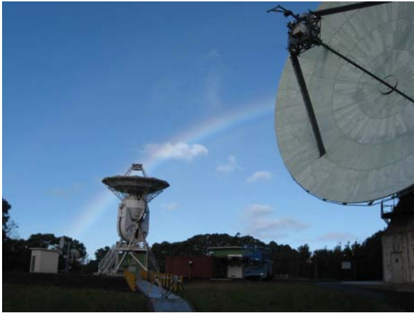
Figure 1. KPGO VLBI 20-m antenna (right) with the old NASA USB 9-m antenna in the background.
