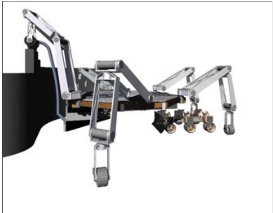
The Microwave Sinterator Freeform Additive Construction System (MS-FACS) uses the ATHLETE mobility system as a positioning system.
