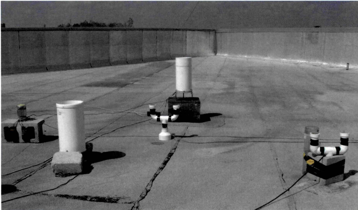
Figure 19. Rainfall measurement test site on the roof of the Engineering Building, UCF, Orlando, FL. Far left is a Joss disdrometer; center and far right are dual-head experimental UCF disdrometers. The large cylinders are tipping buckets. The Joss and tipping buckets are courtesy of NASA Goddard Space Flight Center. In situ calibration of the UCF disdrometers has previously been accomplished via attached tipping buckets which are multiplexed with the disdrometer audio signal.
