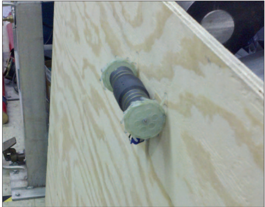
DROP has the ability to climb vertical surfaces, including porous surfaces like wood, using microspine hooks.
