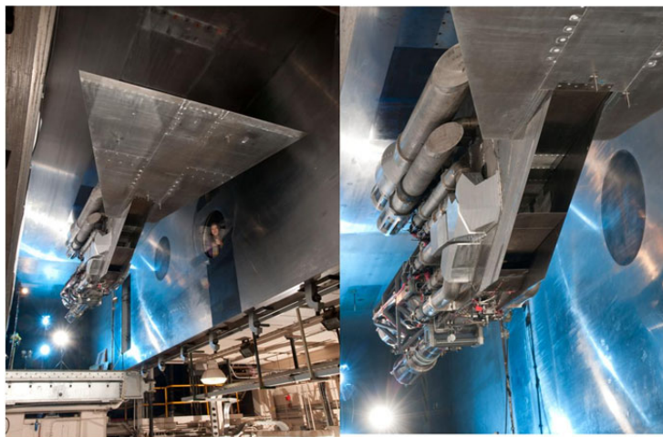
Figure 4.—CCE-LIMX installed in the NASA 10×10 SWT.
