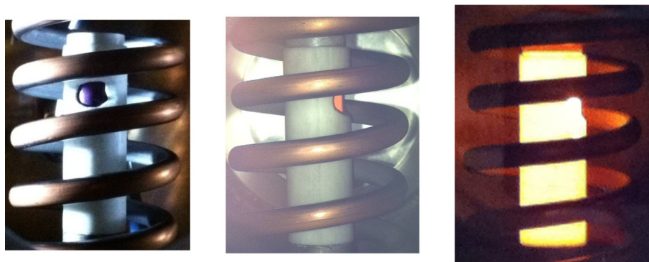
Figure 30. Alumina insulator radiating heat from enclosed sample during test.
