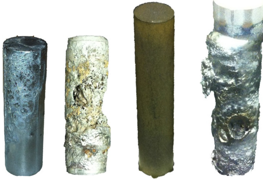
Figure 8. W-Re-HfN samples, before testing and after failure.
