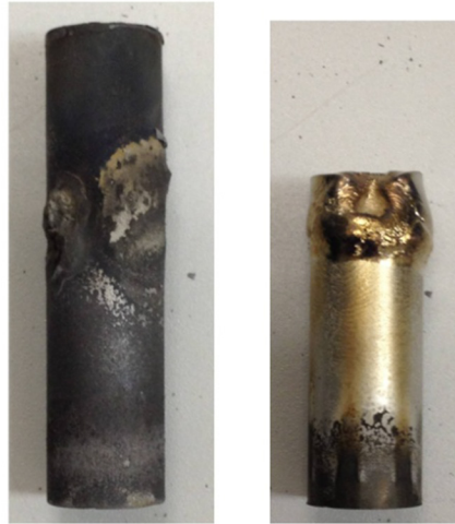
Figure 31. Stainless steel samples after hydrogen tests.
