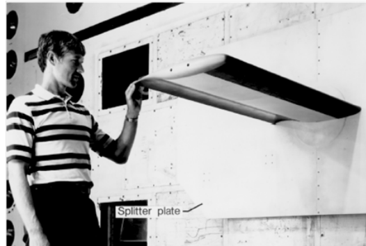
Figure 3. RSW, mounted in the wind tunnel.
