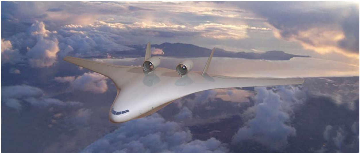
Figure 1. Boeing artist rendering of the Efficient Low Noise HWB 15 (N2A) aircraft freighter concept designed by Boeing Research and Technology to meet simultaneous goals of 25% fuel burn reduction compared to a present day aircraft and 42 dB cumulative noise reduction below Stage 4.
