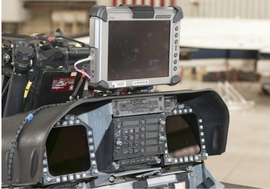
Figure 5. The MDot display mounted in the rear cockpit of F-18B tail number 852.
