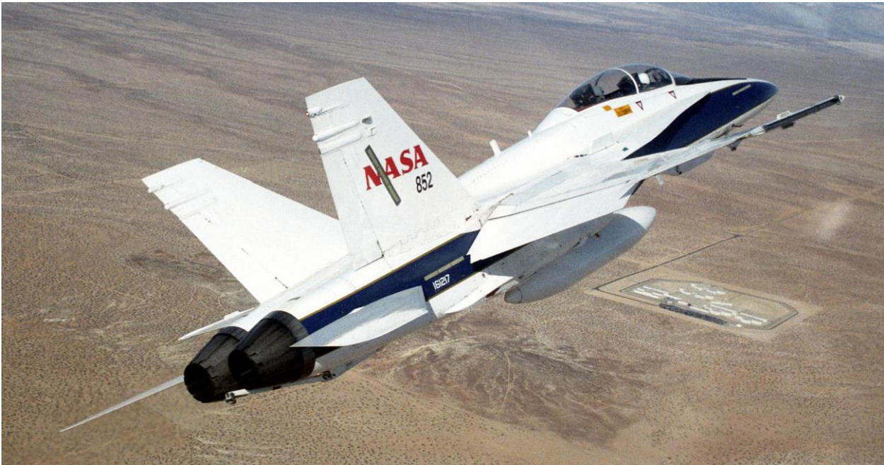
Figure 3. The F-18B airplane, tail number 852, with the centerline fuel tank installed.
