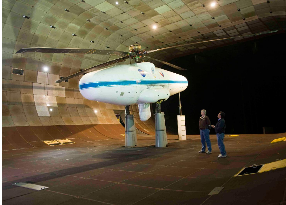
Figure 1. UH-60A Airloads rotor mounted on Large Rotor Test Apparatus in 40- by 80-Foot Wind Tunnel.
