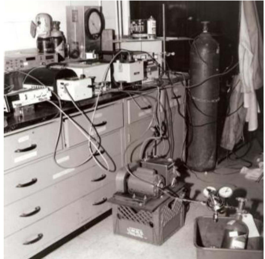
Purifier plumbing, showing vacuum pump used to evacuate cell, and gas bottle used to load cell
