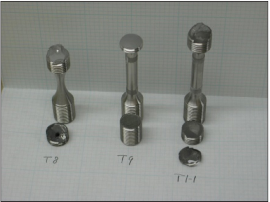
Unanticipated Sample Failures Indicating Notch Sensitivity in Hydrogen
