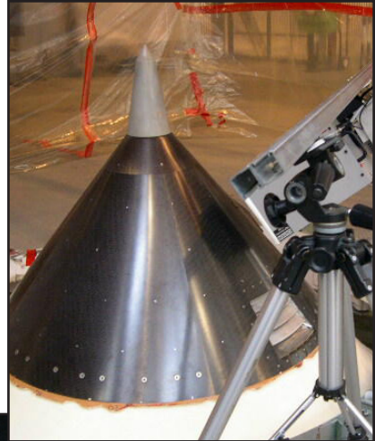
Infrared Thermography of the External Tank Nosecone
