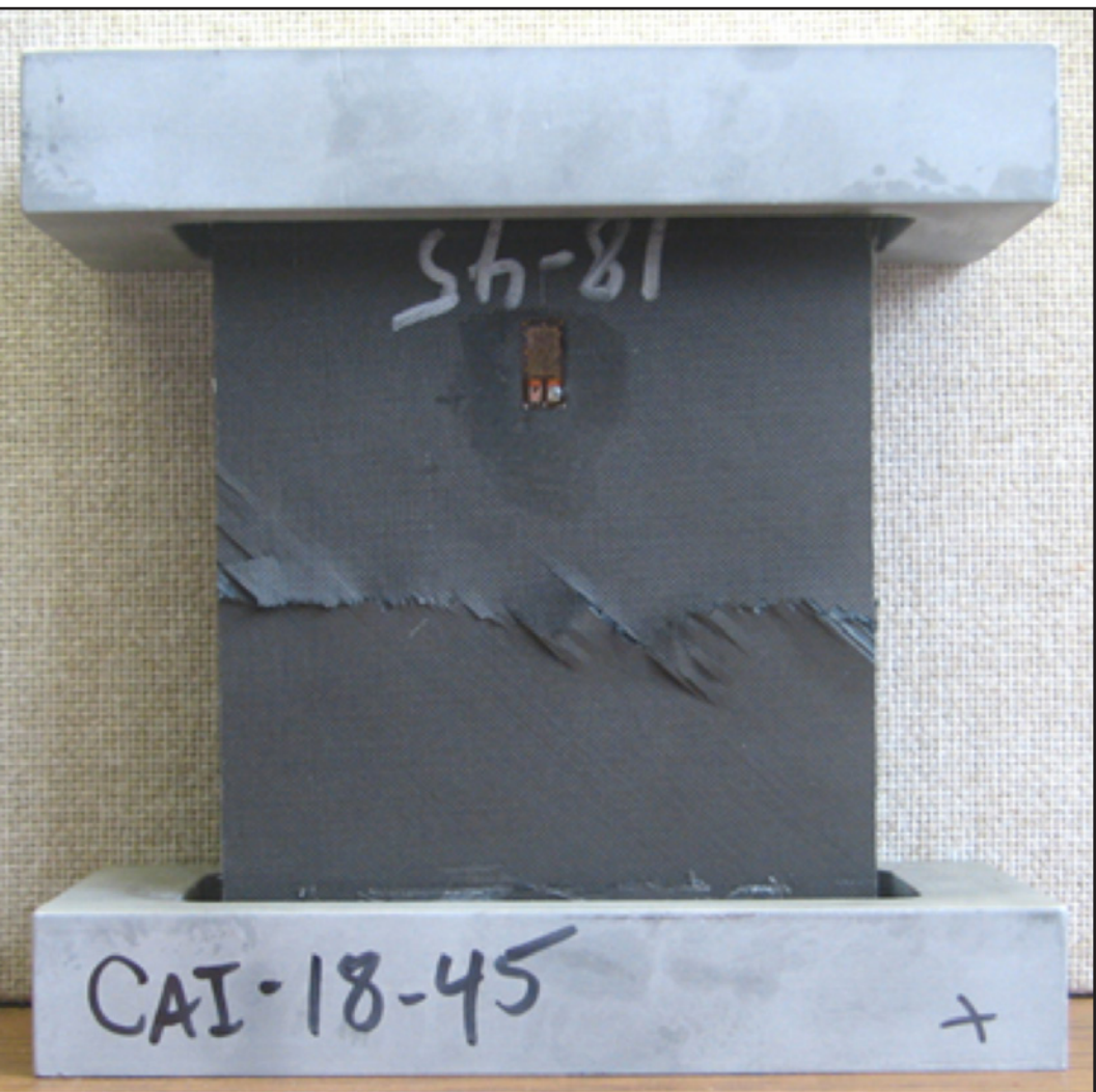
Failed Compression-After-Impact Specimen
