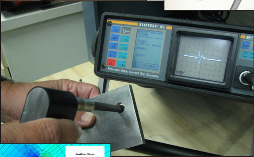
Eddy Current Testing of a hole
