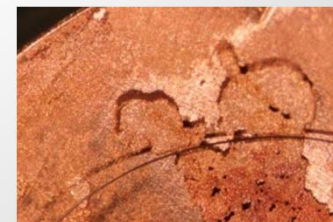
Micrographs of copper electrode and copper flakes recovered from electrode.
