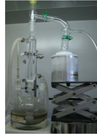
Water extraction from dissolving regolith simulant in acidic IL
