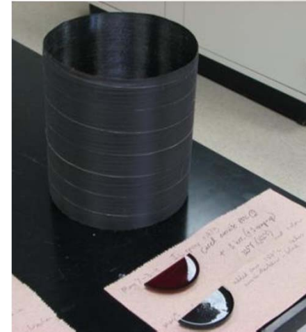
Wound and cured IL epoxy/carbon composite
