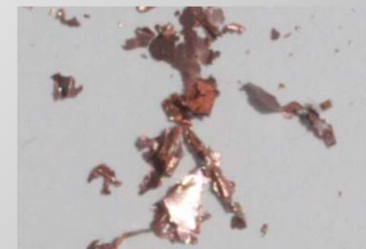
Micrographs of copper electrode and copper flakes recovered from electrode.
