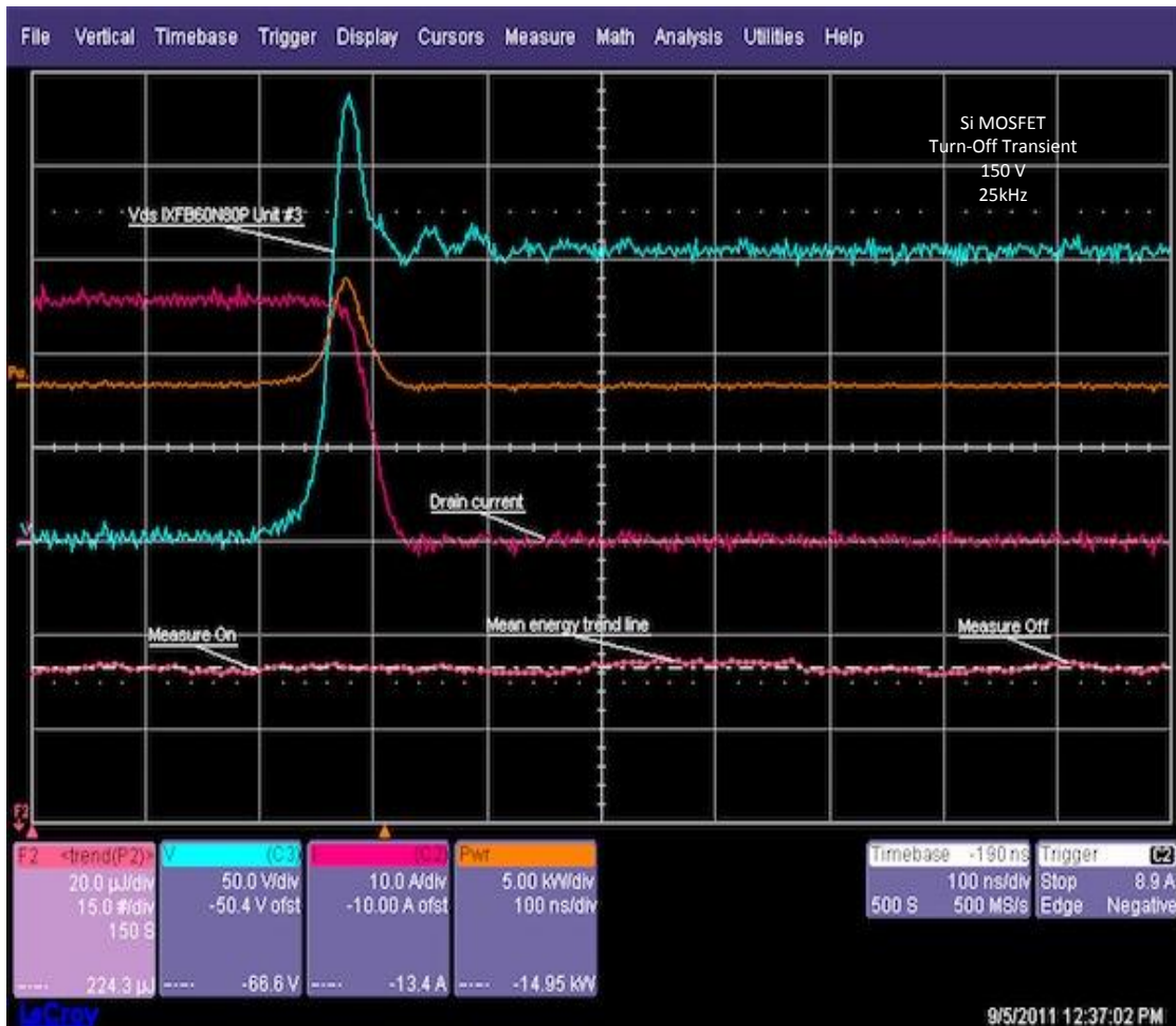
Figure 8. Scope capture of SiC MOSFET turn-off transient at 150V and 25kHz.
