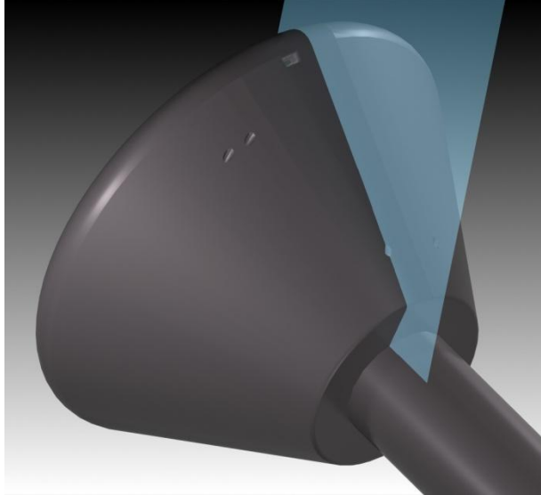
Figure 4: ViDI rendering of the capsule model with simulated laser sheet.
