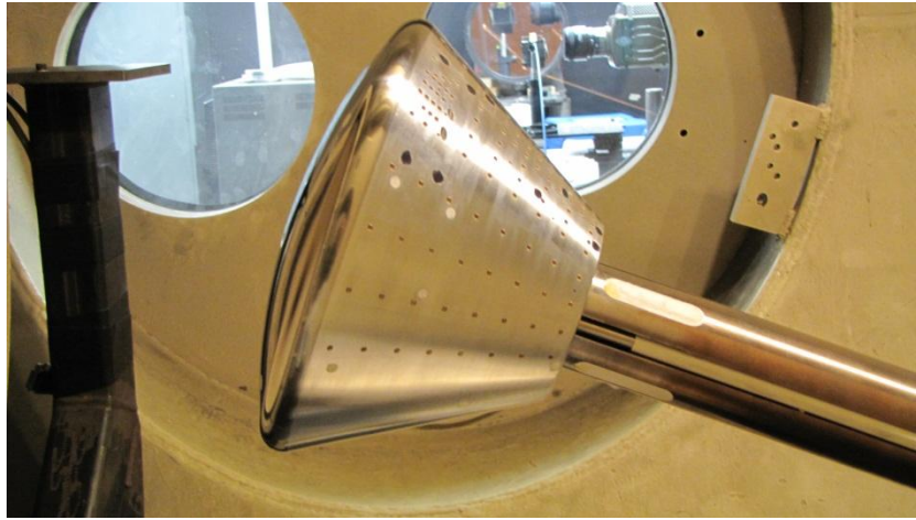
Figure 2: Photograph of the capsule model installed in the test section of the LENS-I reflected shock tunnel.
