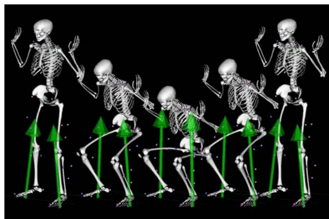
Fig 1: Subject motion and ground reaction forces for the normal ARED squat trial as produced by model scaling, inverse kinematics, and inverse dynamics in OpenSim.
