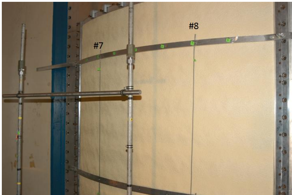
Figure 14. Microphone placements on reverberant side, room modes test. Microphones 1" away from panel.
