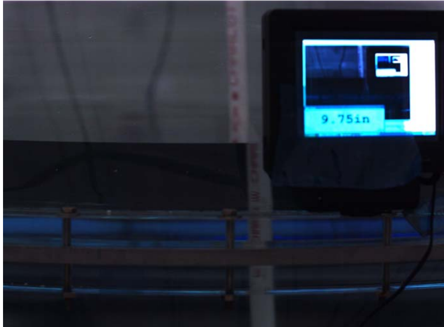
Figure 5: Video Calibration Image. The dark strip in the center of the picture is the water line, just above the upper flange of the Ares I US LOX tank model.
