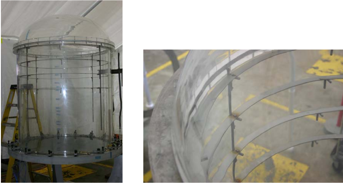
Figure 2: Anti-Slosh Flat Ring Baffles in the Ares I US LH2 Tank Model.
