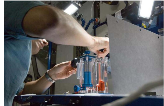
Astronaut Joe Acaba adjusting the vane angle during a recent CFE-2 Vane Gap 2 (VG2) experiment run on ISS (August 10, 2012)
