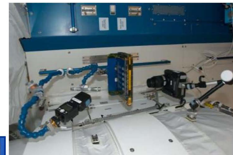
BCAT experiment using the seat track setup in the Japanese Experiment Module
