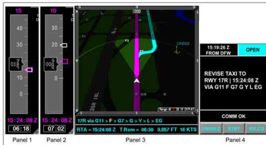
Figure 1 PFD: on straightaway (panel 1), and in turn (panel 2). TND: pending taxi route change with preview information in cyan (panel 3). DataComm: pending taxi route change (panel 4).
