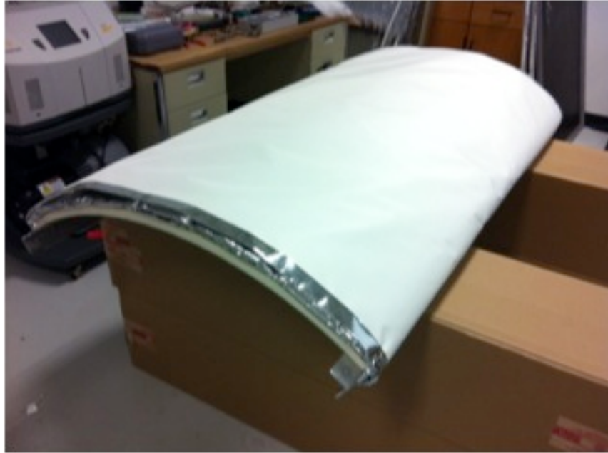
Figure 5. Outer MLI blanket with Beta cloth cover.
