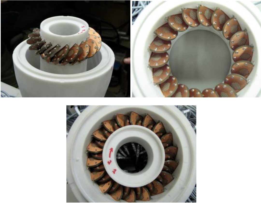
Figure 6.—Actuators Installed in Rapid Prototype Model.
