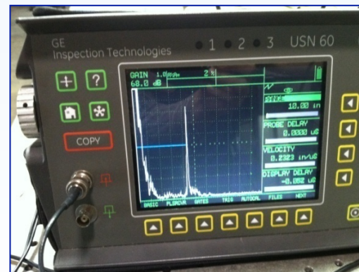
Surface wave ultrasonic NDI technique
