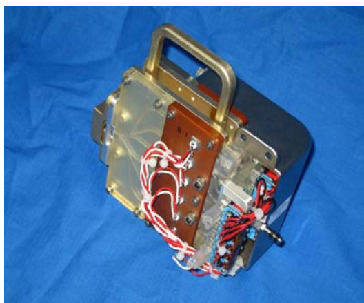
Figure 3: Photograph of a partially disassembled Thermal Precipitator Module with the inlet manifold exposed on the left, the hot wire leads in the red Vespel block in the middle and the outlet valves on the right. The drawing on the right displays the position of the hot wire above the TEM grid with the air flow passing over both. The heated wire drives aerosol particles onto the grid via thermophoresis.
