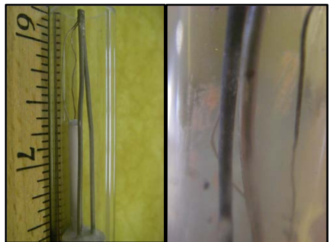
Figure 23. Image Comparison of Catalyst Before and After Test Series. Note the separation and linearity in former and helical shape in after and different scales.
