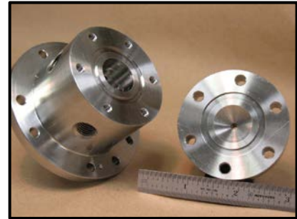
Figure 18. Image of Main Igniter Body with Nozzle Removed.
