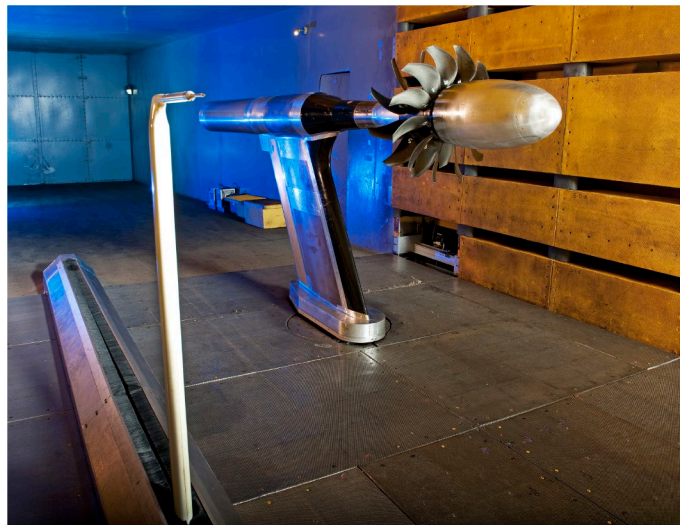
Figure 2.—Model scale F31/A31 historical baseline blade set shown installed in the NASA 9- by 15-foot wind tunnel (2010). The front rotor of F31/A31 has 12 blades and its aft rotor has 10 blades. Traversing inflow microphone system used for sideline acoustic pressure measurements is visible on the left.
