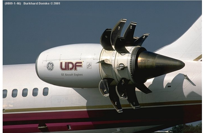
Figure 1.—Top: GE/NASA Unducted Fan (UDF) model installed in NASA wind tunnel (1985). Bottom: GE UDF engine demonstrator installed on the MD-80 testbed aircraft (1987). UDF had equal blade counts, eight each on the front and aft rotors.
