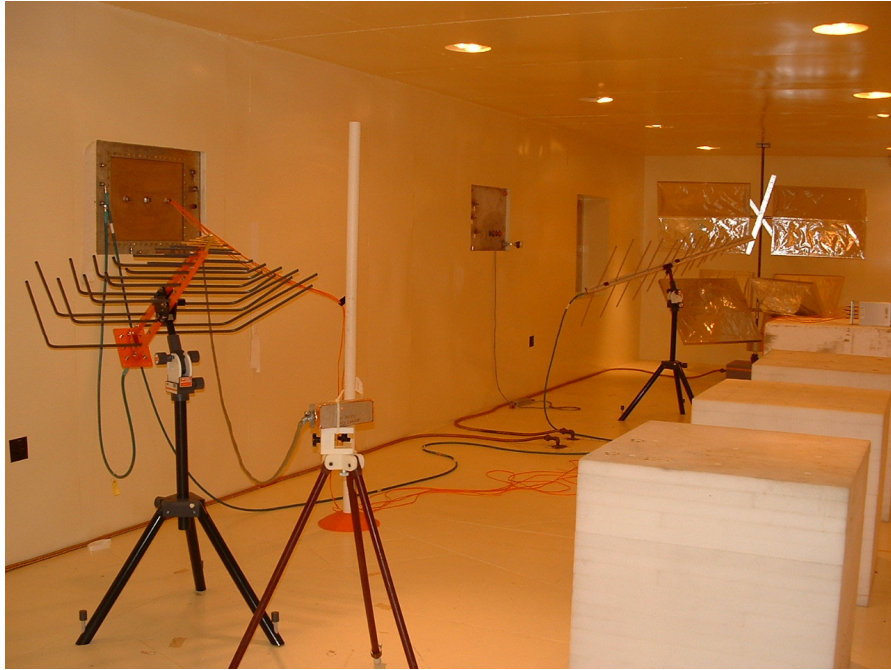
Figure 3: Photo of Reverberation Chamber A taken from the front of the chamber
