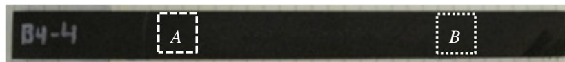
FIGURE 4. Experimental data was collected at two locations, designated A and B , on the composite microcrack sample, designated ‘B4-4’, (with a transducer placed at the centers of the white squares shown in the image). Correspondingly, microCT data for the regions indicated by the white squares was read into the EFIT simulation for comparison to experiment. A-scan comparisons are shown in figures 5-6.
