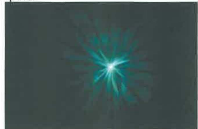
1 st optical image from XACT optics FWHM \sim < 1 arcmin
