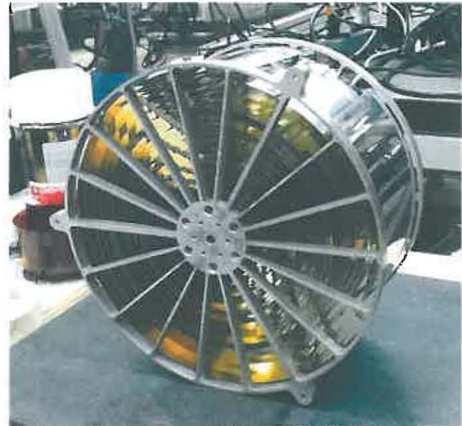
1 st partial assembly of XACT optics
