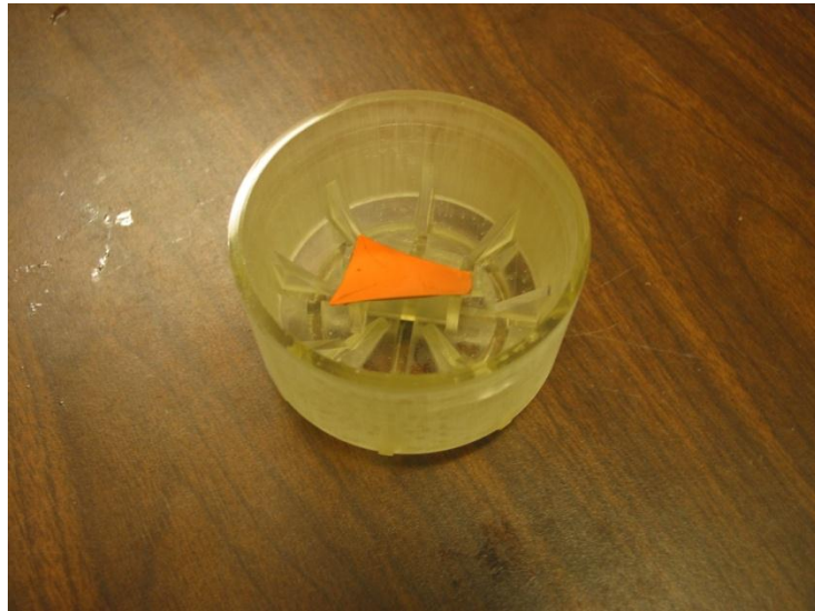
Figure 2.b. Stage 2 blade mounted in sabot.
