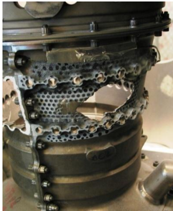
Figure 5. Uncontained impact with no blade exit.
