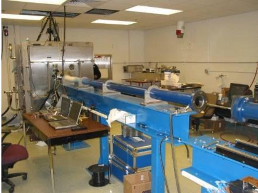
Figure 1.a. Large Vacuum Gun at the NASA GRC Ballistic Impact Facility.
