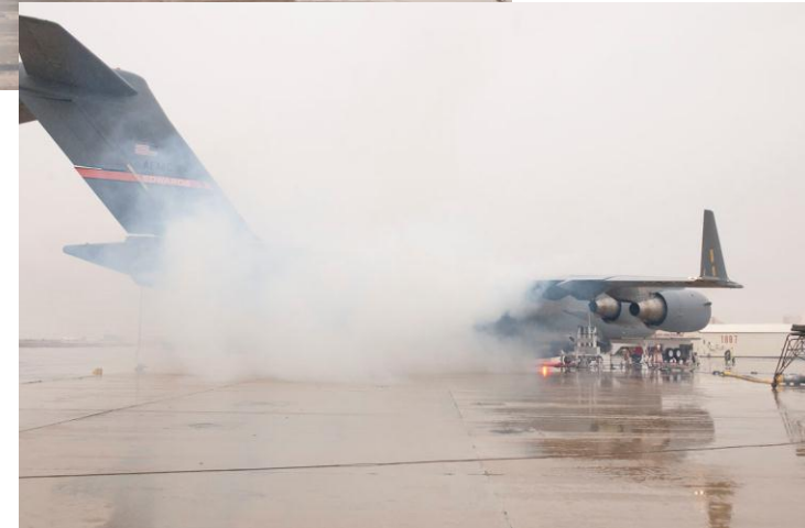
Preservation oil burn-off!
