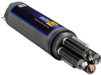
Figure 5: YSI 6600 multi-parameter water quality logger sonde. Note the sensor port cleaning brushes. The manufacturers estimate the sensors will remain calibrated for up to 3 months in pristine alpine waters. The sonde can also operate by itself using its own data-logger and batteries
