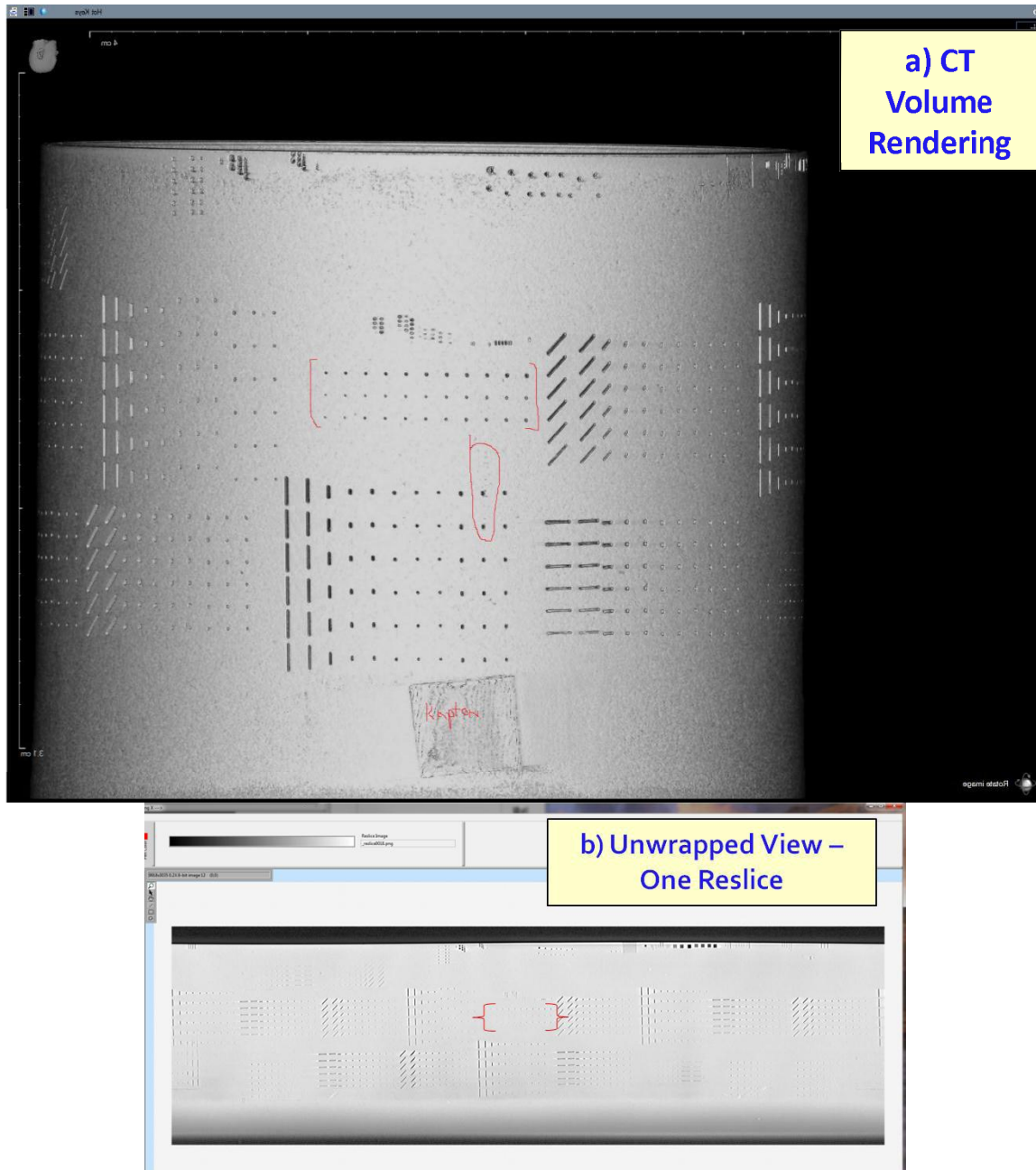
FIGURE 5. a) CT volume rendering and b) one unwrapped reslice for heater head sample with machined-in flaws. Brackets surround one flaw pattern that most closely conformed to specification.
