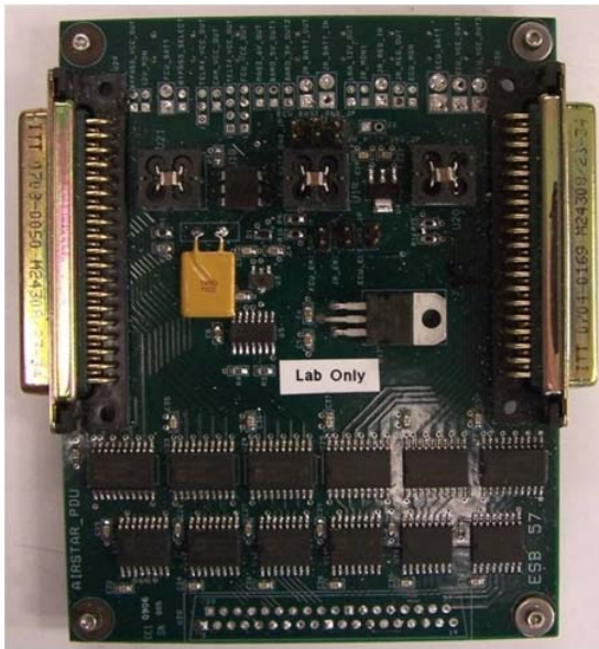
Figure 10. Power Distribution Unit PCB
