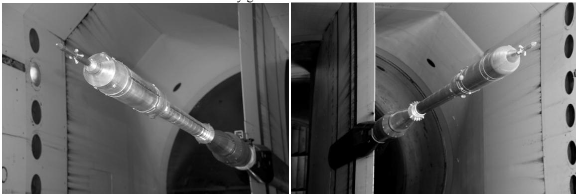
(a) Ares I-X (b) Ares I Figure 1. Rigid Buffet Models installed in the TDT test section.
