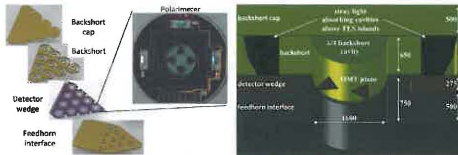
Fig. 2 (Color online) Left : Individual components of a 10-pixel polarimeter array stack. Right : A cross-section, angled model of the OMT in CWG cavity created by the polarimeter array stack. Dimensions are in microns
