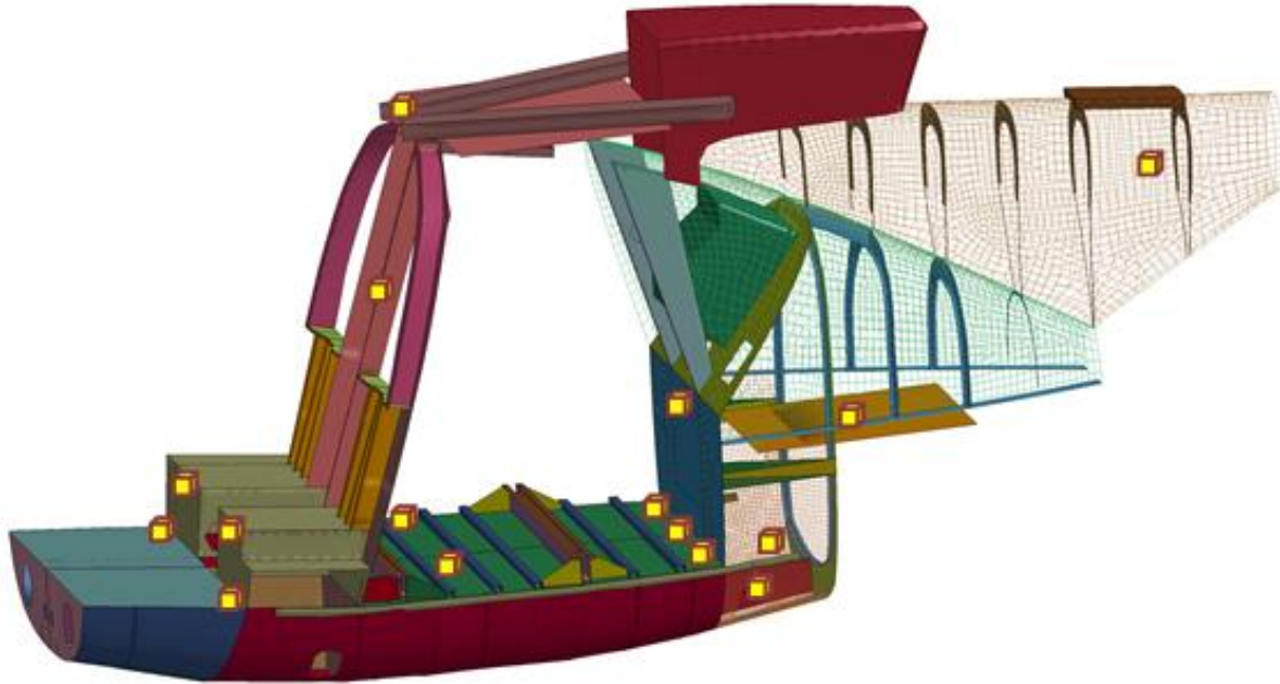
(c) Calibration sensor locations.
