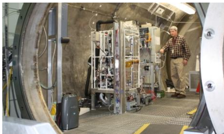
Figure 4. E-Chamber for integrated ARS and EMS testing. Functional demonstration will be accomplished via a three-level testing protocol.
