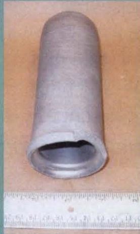
Refractory metal casting for heater head fabrication
