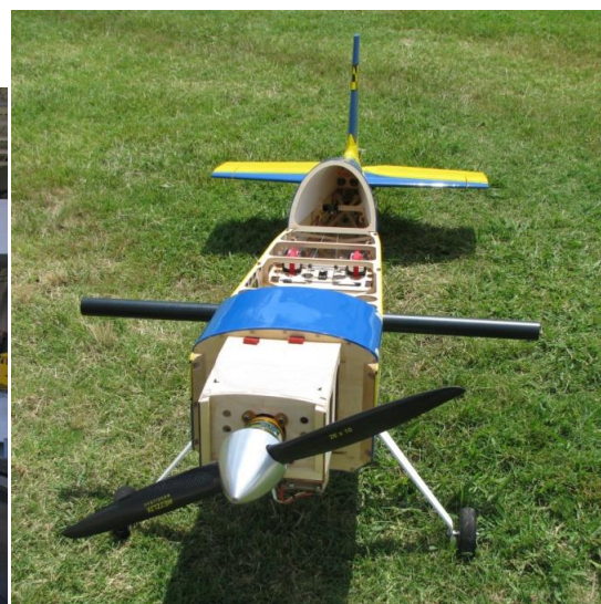
Figure 10: EDGE, left, and with wing support tube showing and wings removed, right
