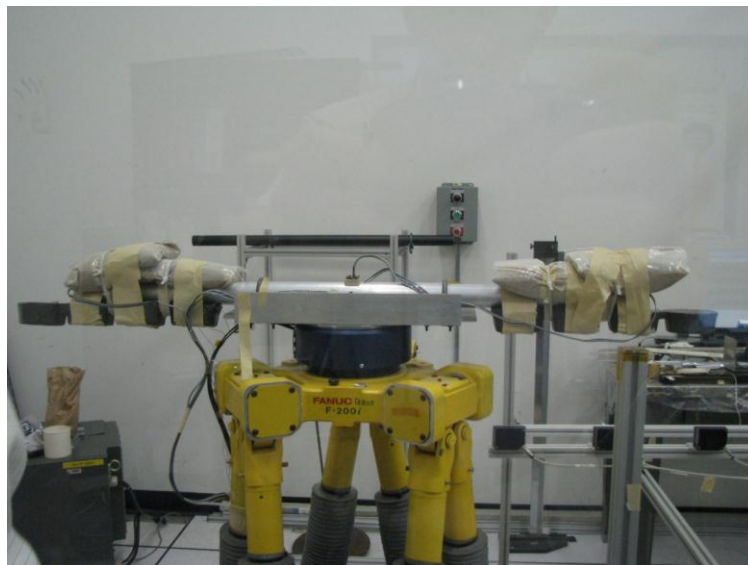
Figure 9: Aluminum tube used for crack detection
