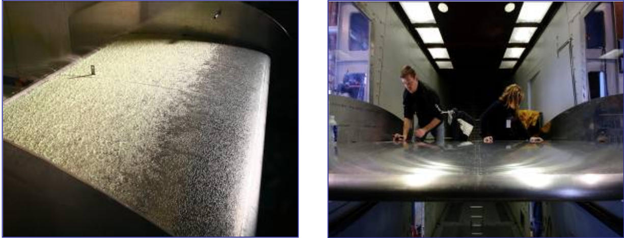
Figure 16.—Photographs of thin, high-performance wing model installed in the NRC PIWT facility.
