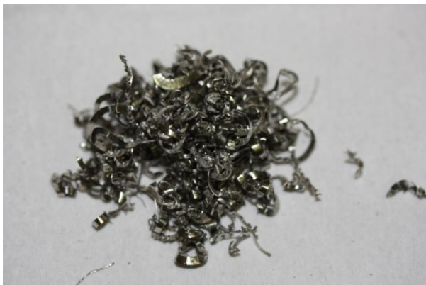
Figure 10. Nickel shavings from solid nickel rod (Ni-Sh).
