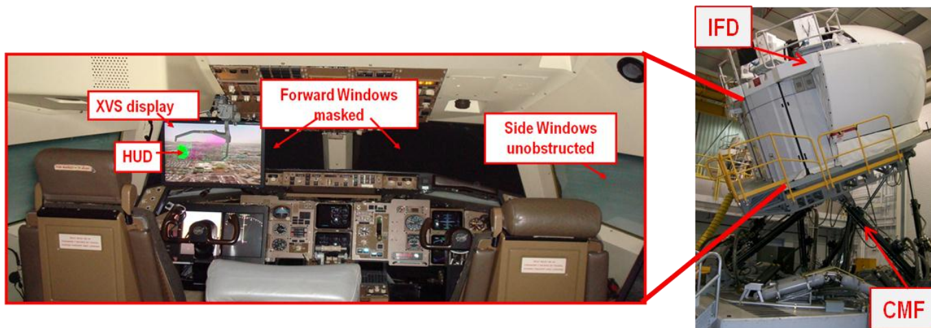
Figure 2. IFD Simulator with HUD, XVS Display (interior view) and CMF with IFD (exterior view)
