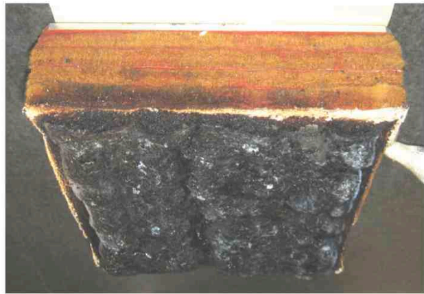
Figure 24a. Post-test cross sections and oblique view of sample 3028 tested at condition C for 60 seconds.
