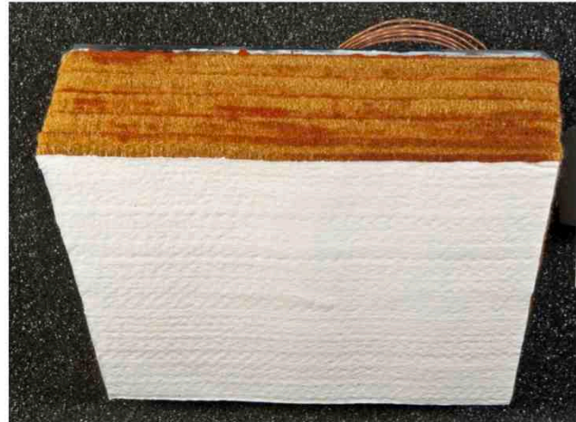
Figure 4. Diagram and pre-test photo of bonded multilayer FRSI test specimen.
