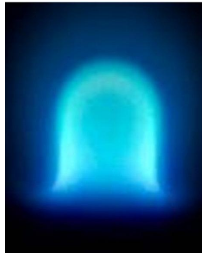
Figure 7. Image of a lifted flame of 50% propylene in a co-flow of air (at ambient pressure) from an exploratory test conducted on the International Space Station in 2009 as part of the Smoke Point In Co-flow Experiment (SPICE).
