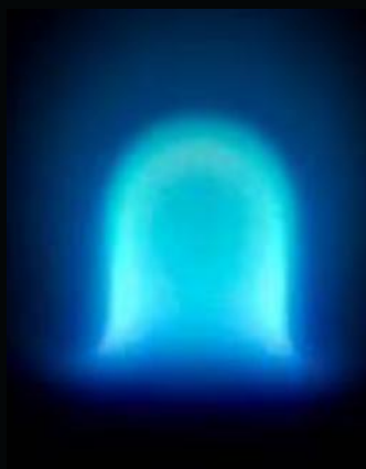
Image of a lifted flame of 50% propylene in a coflow of air (at ambient pressure) from an exploratory test conducted on the International Space Station in 2009 as part of the Smoke Point In Coflow Experiment (SPICE).
