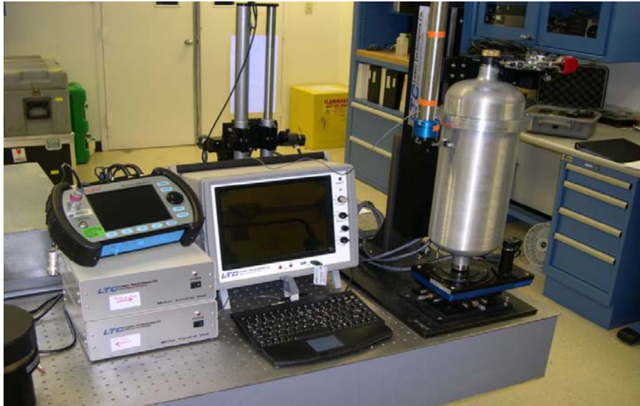
Figure 1. Uniwest US-454A EddyView (top left), LTC Motor Control Unit (lower left), LTC LP-4000 (middle), Probe and Test Article (right)
